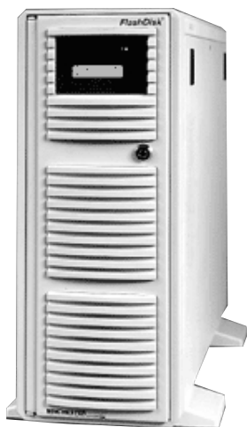
Pedestal Model with 8 or 12 drives provides up to 584 GB of storage.
