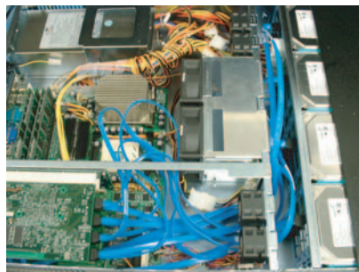
Before 2U system with 12 SATA cables connected
