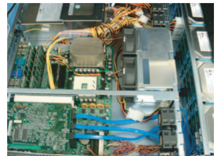
After 2U system with 3 SATA cables connected (includes 3 4-port multipliers on backplane)
